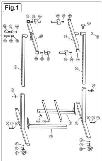
**5.1.** Use original engine mounting bolts or studding, washers and nuts of appropriate size to secure the engine to the stand using supporting frames (21 & 22).
